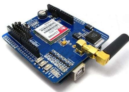
Gbr. 9. Arduino GSM shield
