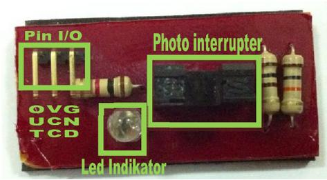
Gbr. 25 Rangkaian sensor *rotary encoder*.
