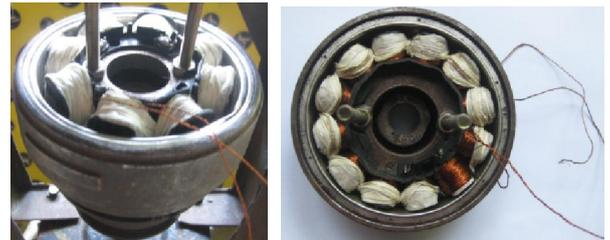
Gbr. 10 Rotor Generator Fluks Radial Satu Phasa
