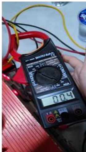
Fgr.8 The results of the current value through measurements using a Clamp Meter
