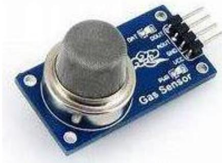
Gambar 5. Sensor Gas (MQ2)
