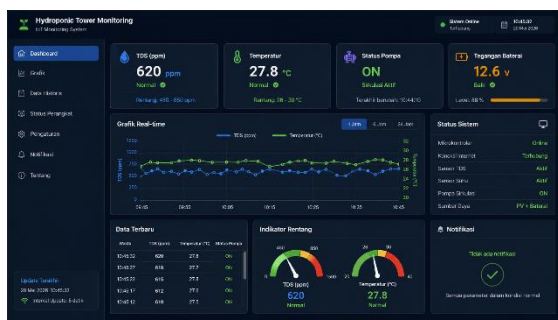
Gambar 4. Tampilan Dashboard Monitoring TDS dan Temperatur
